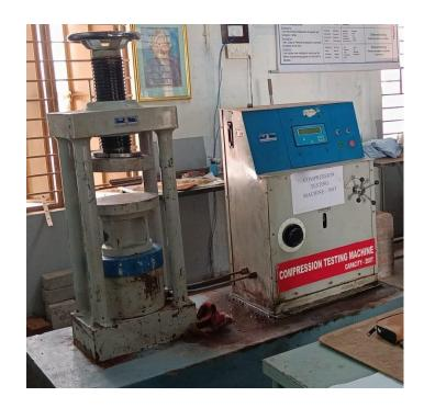
Universal Testing Machine (100 tonne)
